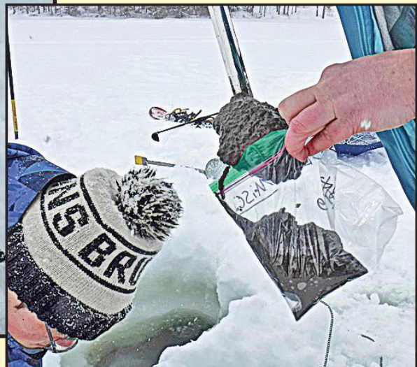
Spooning the sediment into a labeled baggie to be analyzed at Colby College.
